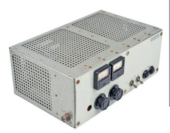
General view of 300B RF amplifier. The left hand part was taken by the RF part and the other side by the heavy mains power unit.
