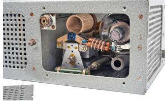
Rear view of 300B RF amplifier showing the QE08/200 valve and RF tank circuit.
